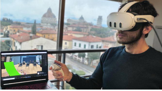
Fig. 2. An example of the experimental set: the participant wears a Virtual Reality headset showing a waiting room that is progressively filled with virtual avatars more and more interacting between each other. The controller's joystick allows a continuous recording of the participant's level of subjective anxiety, represented through a green bar (partially visible in the computer's screen) shown in the periphery of the visual field (the positioning can be manually adjusted by participants to fit their own visual field)
